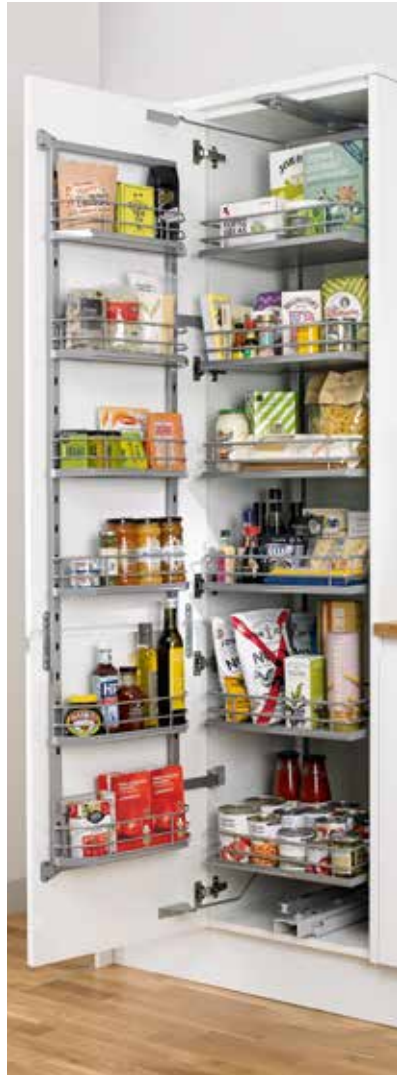
Full-Height Pull & Swing Larder 500mm wide HYH1337 6 pull-out baskets and 6 door-mounted baskets with anti-slip coating, solid base and soft closing runners 3.5kg maximum weight per door-mounted basket 8kg maximum weight per pull-out basket
